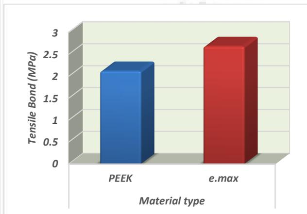
**Figure (4):** Column chart showing the mean values of tensile bond strength for both material groups
