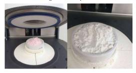
Figure 1: removing the food dye from the ceramic powder
