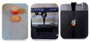
Figure (1) : 2mm thick cervical section ready for fracture resistance test with the universal testing machiene
