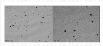
Fig. (1): transmission electron microscope image of AgNPs (orig. mag. x200000).
