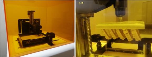
Figure 3 - 3D printer with light protection cover, inside view of printed models
