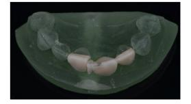
Fig 4: Fractured VRFDP at the connector
