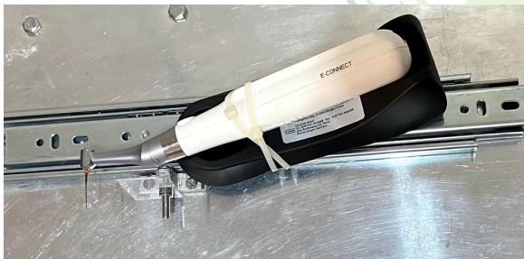
Figure 5: Picture, showing the custom-made device for measuring cutting efficiency of the three rotary systems.
