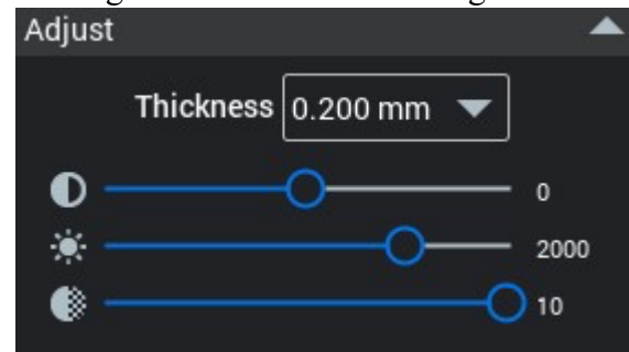
Figure (1): Image display parameters as shown in the software (from top to bottom): Slice thickness, contrast, density (brightness), and sharpness.
