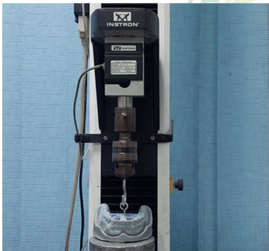
Figure 5: The connection of the circular hook of the overdenture to the metal hook of the universal testing machine during the pull
