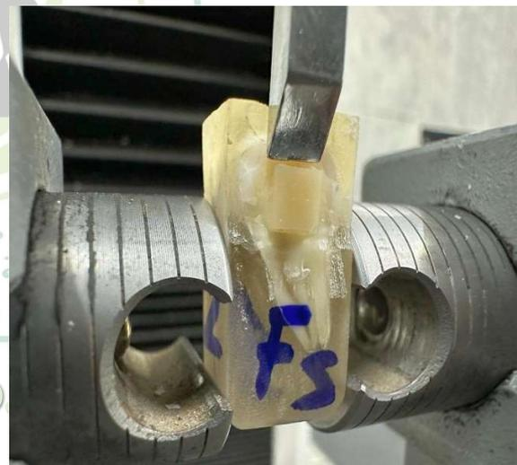
Figure 4: prepared tooth with block cemented and universal testing machine in place
