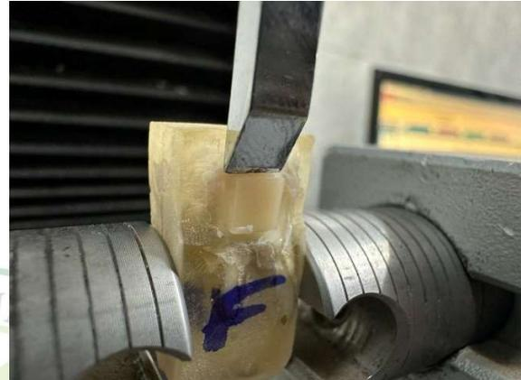
Figure 3: universal testing machine for shear bond strength testing.
