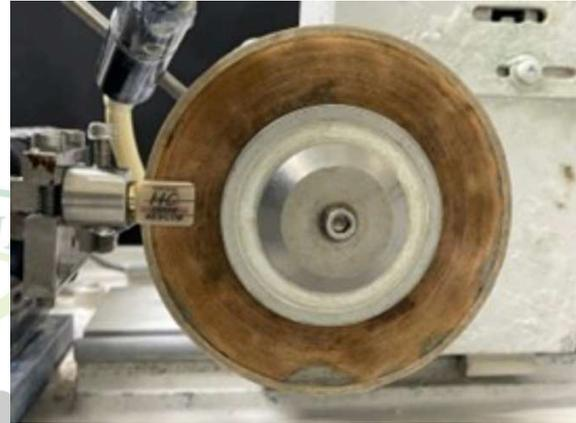
Figure 1: low-speed isomet saw for sectioning the specimens.
