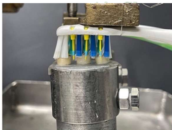
Figure 2: tooth brush head contacting surface of specimens during stroke under vertical load
