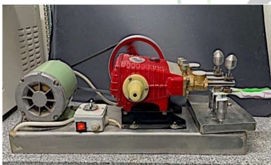
Figure 1: Automatic tooth brushing simulating machine
