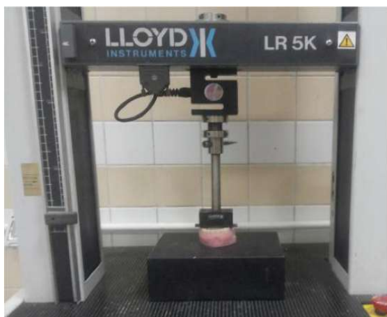
Fig (1): Maxillary denture on the prepared cast placed in the universal testing machine.
