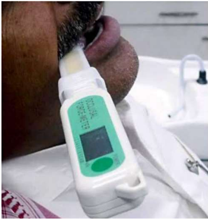
Figure 3: The Load sensor was positioned horizontally at the location of the second premolar and first molar embrasure with the patient seated upright.
