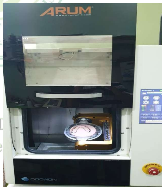
Figure 4: PEEK overdenture base milling.
